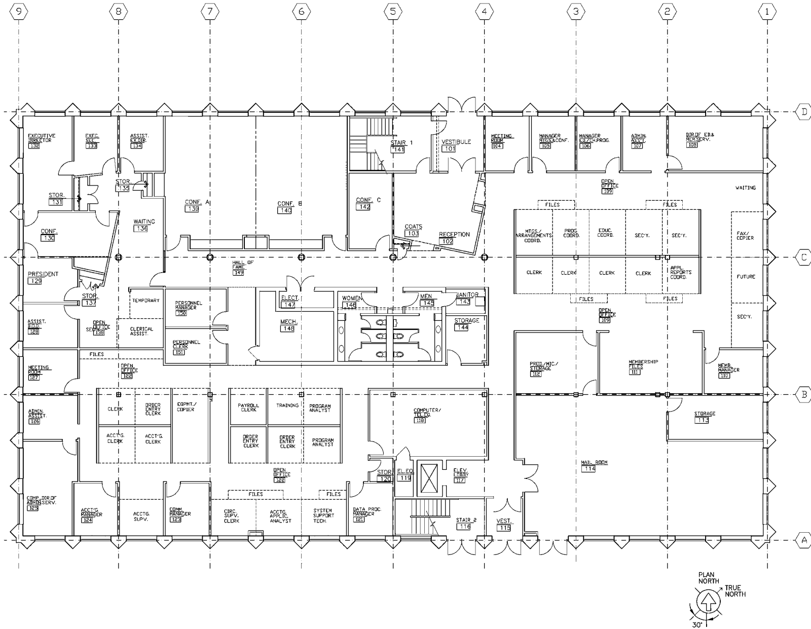
Fig. 23 First Floor Tenant Plan (not to scale)
